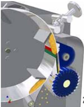
The three dimensional cutting operation with synchronized speeds of the spindles controls the product during the cutting operation and prevents the product from changing direction resulting in an unmatched product uniformity.
