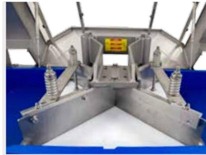
The product to be cut is fed onto a conveyor belt that passes under a vertically moving set of guillotine knives. The distance the belt travels per stroke of the set of knives determines the cutting size, which can easily be adjusted (from 5 to 40 mm) with an external hand wheel.
